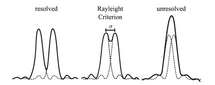
**Resolving power of grating:** The resolving power of grating is its ability to just distinguish two nearby spectral lines with two close wavelengths. If the wavelength of two nearby spectral lines be  $\lambda$  and  $\lambda + d\lambda$ , the resolving power of grating is defined mathematically as  $R.P. = \frac{\lambda}{d\lambda}$ . So smaller value of  $d\lambda$ , we get the larger value of resolving power.
